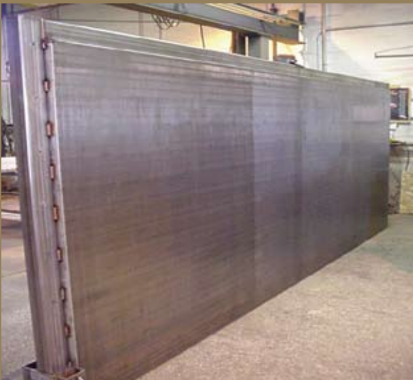
Fish Diversion Screen
